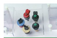
Side feed injector cradle
